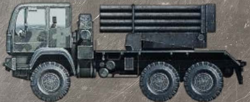
Soviet MLRS – 120mm BM-21 GRAD systems with standard (20km) and long-range (40km) rockets
